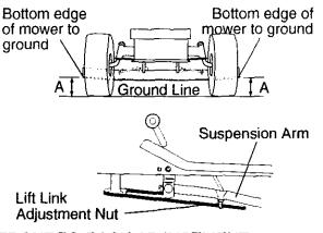
FRONT-TO-BACK ADJUSTMENT IMPORTANT: Deck must be level side-to side. If the following front-to-back adjustment is necessary, be sure to adjust both front links equally so mower will stay level side-to-side.
